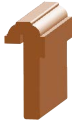
T-Astragal with Weatherstrip Kerf for 2-1/4" Doors 1-1/2 x 3-3/8
